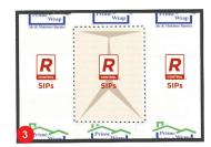
Make and inverted Y cut in the housewrap at rough opening.
