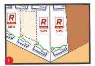
Start with lowest course, 2-3 feet from a corner. Secure Prime Wrap housewrap firmly in place by fastening it every 12" to 18" along the vertical studs using large-headed or plastic cap nail or 1" crown staples.
