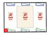
Continue to unroll the Prime Wrap tightly around the structure - covering all door and window openings. While nailing or stapling make sure the fabric is taut against the exterior wall and not sagging. Seal all seams, tears, and cuts with Prime Wrap Sheathing Tape.
