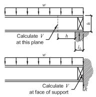
Figure 4.4.5: Design Shear Force
