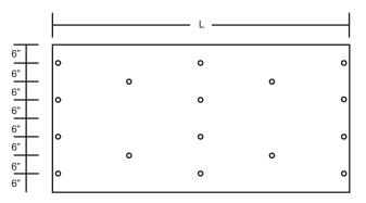
Connection patterns for three span condition
