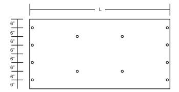
Connection patterns for two span condition
