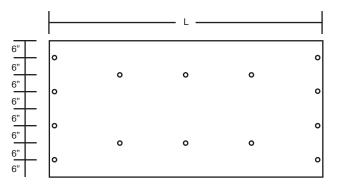
Connection patterns for three span condition
