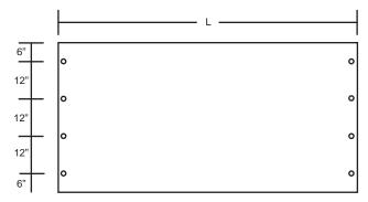
Connection patterns for single span condition
