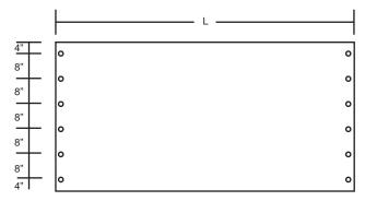
Connection patterns for single span condition
