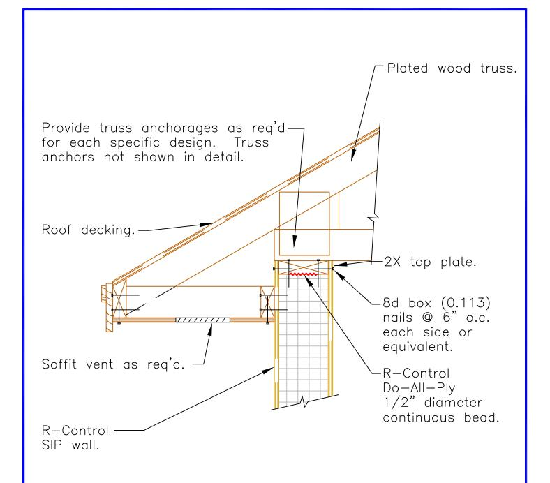
Note: Design member sizes and connections as req'd for each condition and/or project.
