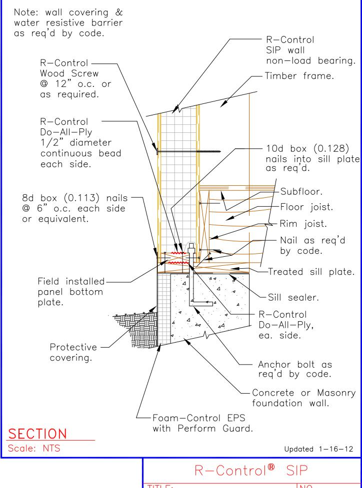
NO. Foundation Framing — Joist SIP-203
