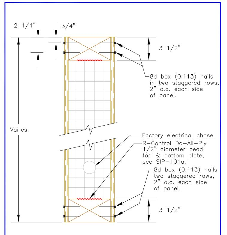
NOTE: OSB facings must be fully supported by foundation system.
