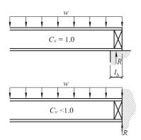
Figure 4.4.4: C<sub>v</sub> Support Conditions
