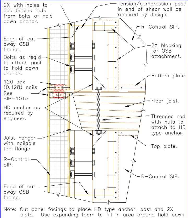
Replace OSB facing and nail to 2X blocking. anchor.
