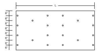
Connection patterns for four span condition
