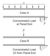
Figure 4.6.2.2: Bearing on Facings
