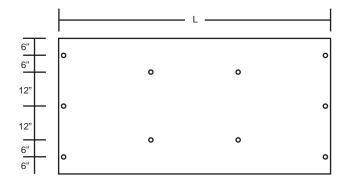
Connection patterns for two span condition
