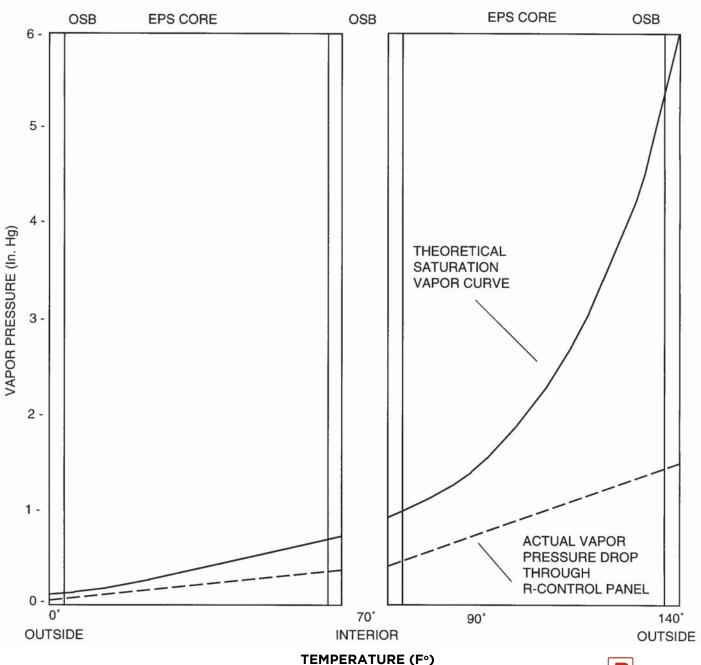
NOTE: Since vapor pressure through the R-Control SIP does exceed saturation curve, condensation does not occur.
