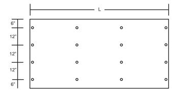
Connection patterns for two span condition
