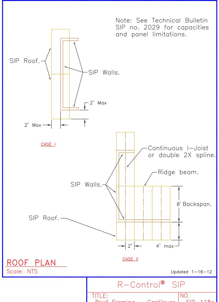
SIP-118a Roof Framing — Cantilever
