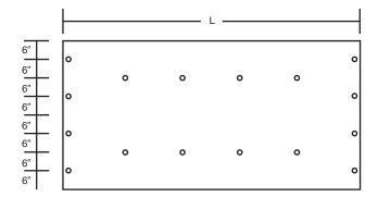
Connection patterns for four span condition
