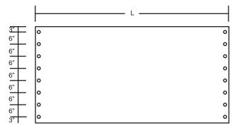
Connection patterns for single span condition
