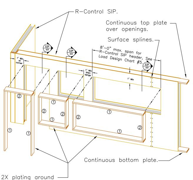
NOTE: Diagram represents headers in a monolithic wall assembly. Splines may occur above & below openings. Minimum panel dimension of 12" must be maintained over openings.
