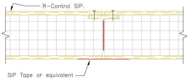
SIP Tape or equivalent vapor retarder located interior or exterior per climate conditions or code requirement.
